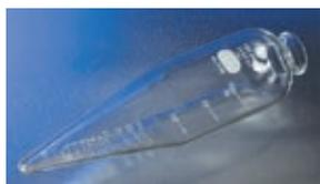
**8190 PYREX Tube, Centrifuge, Oil, Graduated**
