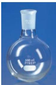
**4321 PYREX® Flask, Boiling, Round Bottom, Short Neck, ⚗ Joint**
