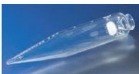
**8160 PYREX Tube, Centrifuge, Oil, Graduated**
