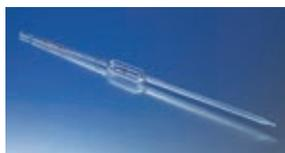
**7103C PYREX® Pipet, Serialized/Certified, Class A, Volumetric, Color-coded, Colored Graduations, To Contain, To Deliver**
