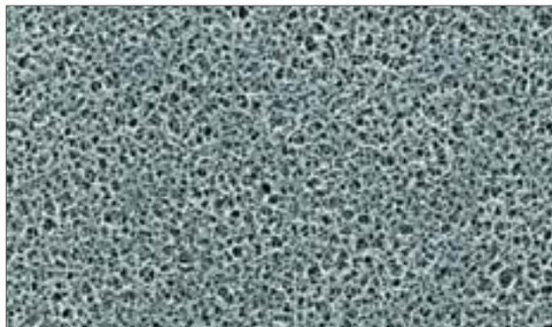
Regenerated Cellulose Membrane (Type RE 55, 0.45 µm)
