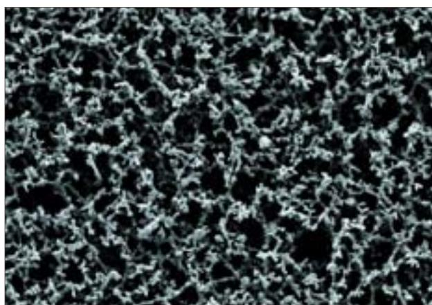
Cellulose Acetate Membrane (Type ST 68, 0.8  $\mu\text{m}$ )
