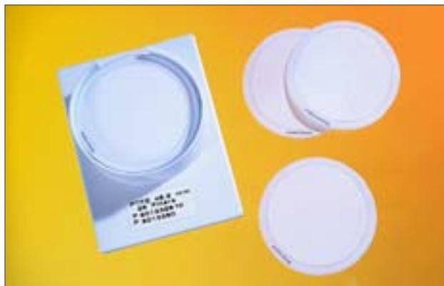
Any filter manufacturer or vendor who sells or offers to sell filters specifically identified for use with this PM 2.5 reference method shall certify that the required number of filters from each lot (0.1% or 10, whichever is greater) of filters offered for sale have been tested as specified for the following tests and meet 90% of each of the design and performance specifications:
