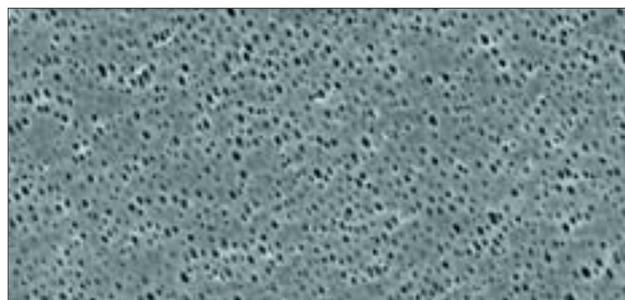
*Polyamide Membrane (Type NL 17, 0.45 µm)
